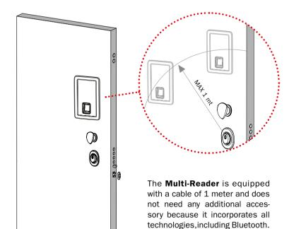
The **Multi-Reader** metal box\* is also available and this is useful in case it is necessary to cut the internal metal panel of the door to fit the Multi-Reader. The metal box must be welded to the metal panel, cut to the size of the box. With these dimensions the Multi-Reader works correctly with all the available technologies.
