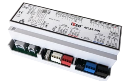
ATLAS PLUS DIN WITH POWER OVER ETHERNET (configurable as Master or Slave)
