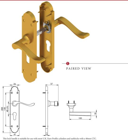
This lock handle is suitable for use with most U.K. Euro Profile cylinders and sashlocks with a 48mm CTC.
