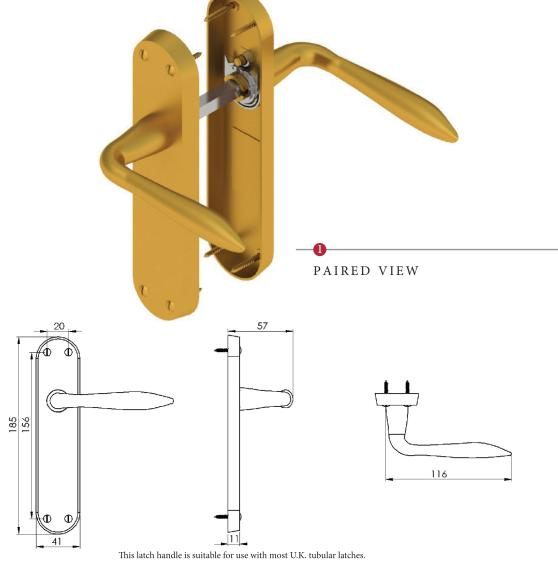
For a new door installation we would recommend using our York standard tubular latch from the list below. Please select the size and finish required.
