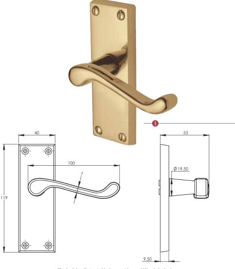
This latch handle is suitable for use with most U.K. tubular latches. For a new door installation we would recommend using our York standard tubular latch from the list below.
