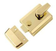
**Deadbolt**: A bathroom bolt is a locking mechanism that uses a solid metal bolt which extends into the door frame to lock the door for privacy. It is designed to be locked from the inside without a key. It cannot be pushed back without the correct internal control (thumbturn or emergency release). Suitable for bathrooms, and a privacy setting rather than security.
